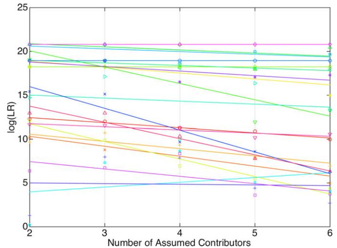
FIG. 3—Information with excess contributors (two-person mixtures). In separate computer runs, TrueAllele assumed 2, 3, 4, 5, or 6 unknown contributors and inferred  $\log(\text{LR})$  match statistics. For each mixture component, the regression line and data points are shown under these five different contributor assumptions.
