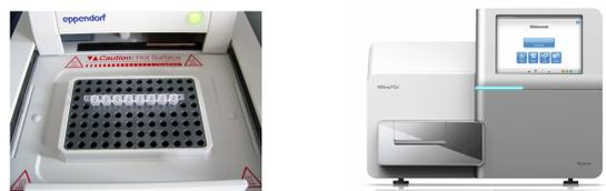
Samples are prepared in the same way as traditional DNA analysis, but using specific NGS testing kits to amplify the DNA samples (top left). The MiSeq FGx Sequencing System (top right, image from [2]) is used to generate the NGS DNA data. NGS DNA data output includes both autosomal STR data (select loci, bottom) and SNPs.
