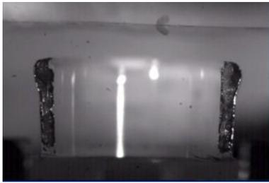
Laser-cut cell falls by gravity into the cap of a 0.2ml PCR tube located directly below the stage
